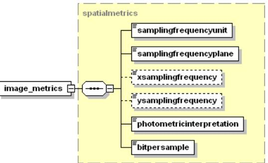
A diagram showing the structure of the 'spatialmetrics' element. It is a container for several child elements: 'samplingfrequencyunit', 'samplingfrequencyplane', 'xsamplingfrequency', 'ysamplingfrequency', 'photometricinterpretation', and 'bitpersample'. The 'spatialmetrics' container is highlighted in yellow. |
