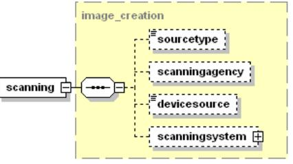
A diagram showing the structure of the 'image_creation' element. It is a container for four child elements: 'sourcetype', 'scanningagency', 'devicesource', and 'scanningsystem'. The 'image_creation' container is highlighted in yellow. |
