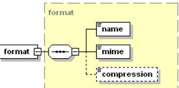
A diagram showing the structure of the 'format' element. It is a container for three child elements: 'name', 'mime', and 'compression'. The 'format' container is highlighted in yellow. |
