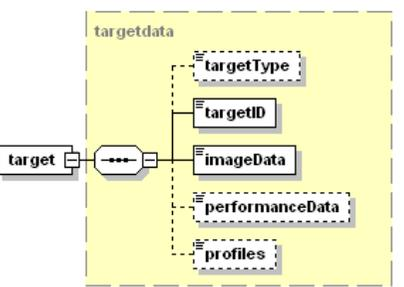
A diagram showing the structure of the 'targetdata' element. It is a container for four child elements: 'targetType', 'targetID', 'imageData', and 'performanceData'. The 'targetdata' container is highlighted in yellow. |
