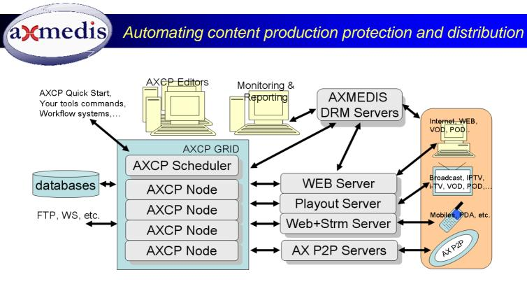
AXMEDIS tools (AXMEDIS P2P, AXCP, AXMEDIS DRM, AXMEDIS COPOP, etc.) have been designed to satisfy a large set of requirements collected by AXMEDIS Consortium partners and user group AXMEDIS tools are based on modular components which can be reused to set up a large range of different configurations/solutions. They are open to be customized to cover your needs and business ideas. For any issue, please contact AXMEDIS reference person.
