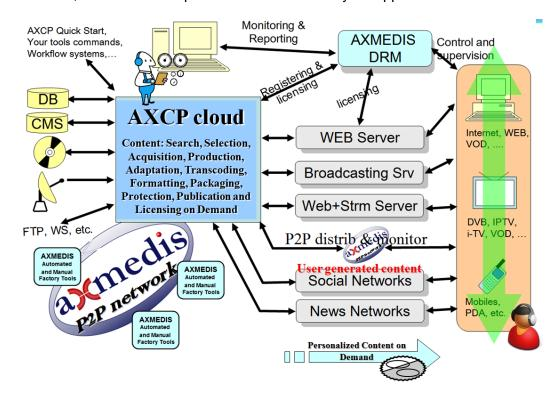
AXCP is an integrated solution to set up scalable architectures of cloud computing, industrial grid, which can be functional to several kinds of applications:
